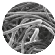
Front view of the conventional polyester filter enlarged 100x
