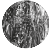
Front view of the conventional polyester filter enlarged 50x
