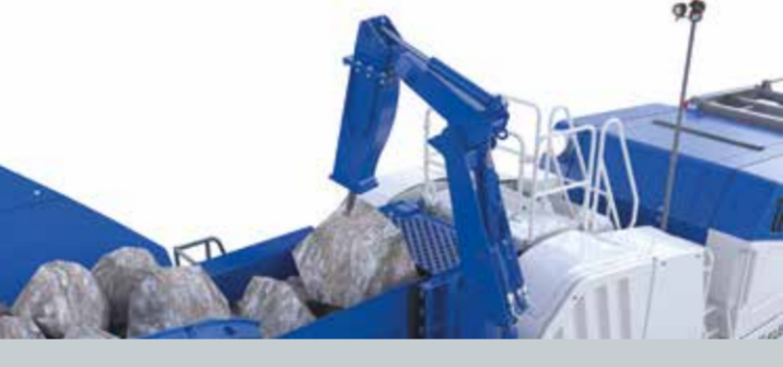
Rigid and foldable side discharge conveyor + available - discharge height of 3.5 m
