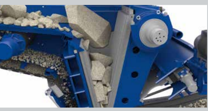
Flattened transition, highly raised crusher jaw
